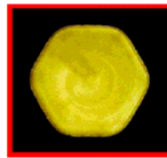
Hexagonal core/clad shaped fiber
