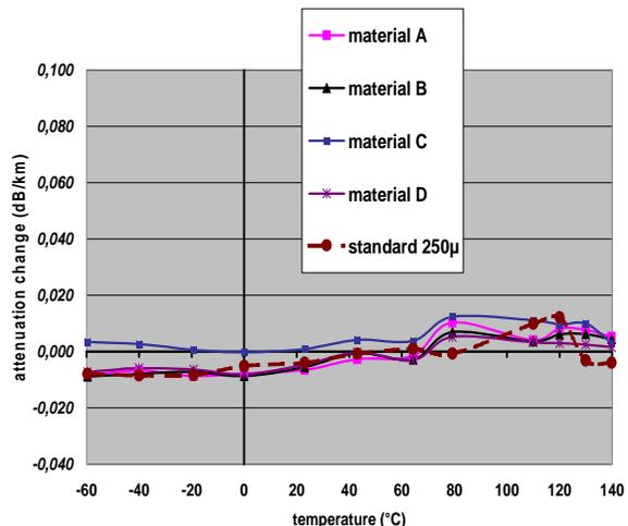
**Figure 8. Attenuation change for 500µm fibers with different upcoated materials with sliding layer**
