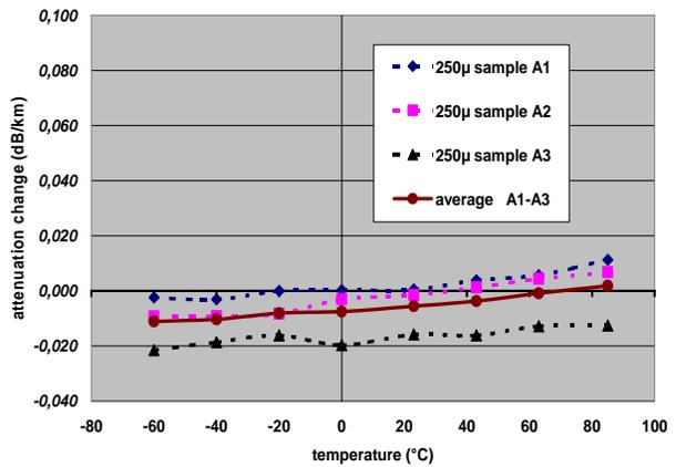
Figure 6. Variation of measured attenuation change for standard 250µm fibers
