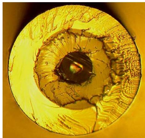
**Figure 3. Typical cross section of a 50µm core Multimode fiber with an originally applied 500µm coating**
