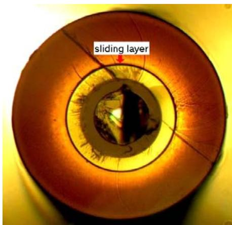
**Figure 1. Typical cross section of an upcoated fiber with a thin sliding layer**
