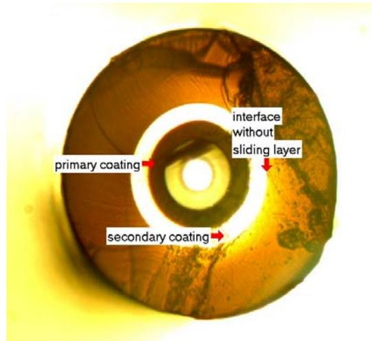
**Figure 2. Typical cross section of an upcoated fiber without a sliding layer**
