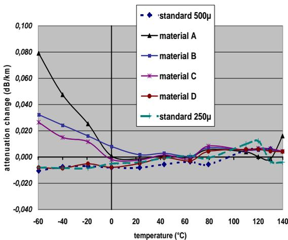
**Figure 7. Attenuation change for 500µm fibers with different upcoated materials without sliding layer**
