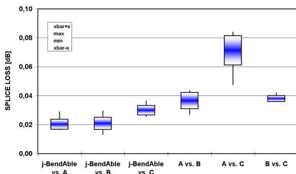
The experiments have been conducted by use of a commercial splicing tool and by applying the standard multimode program of the splicing tool.
