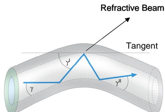
The reason: higher modes are not being guided through the fiber parallel to the fiber’s axis but in a specific angle. Bending
