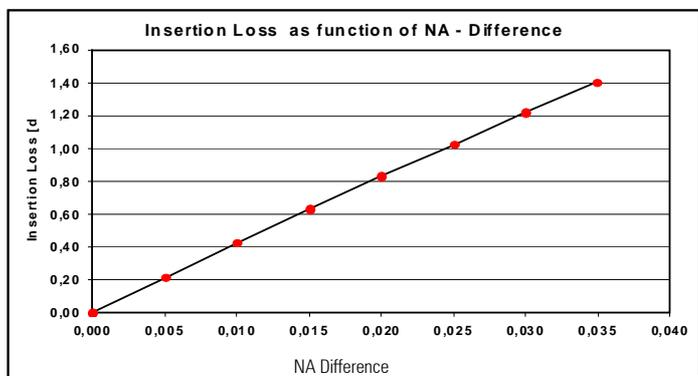
One requirement in fiber design demands to meet the specifications for core diameter and NA as closely as possible. This e.g. means to choose the appropriate trench position and design in the profile, a design parameter with very significant effect on the splice loss.
