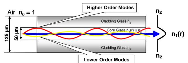
What happens in case of bending the fiber? To explain it in a very simplified way: the fiber loses energy, the attenuation increases.
